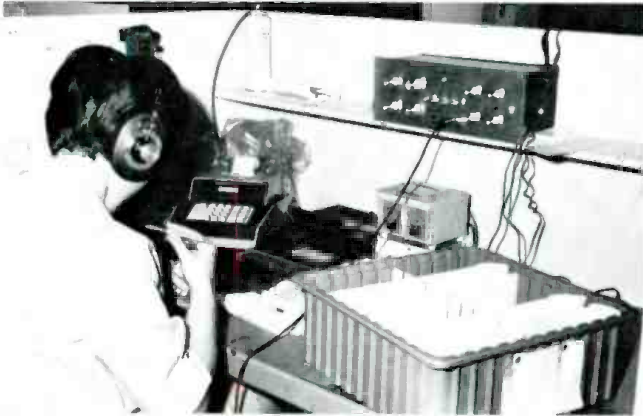
Process quality control station for mechanical checks of loaded cassettes and eight-track tape cartridges.
